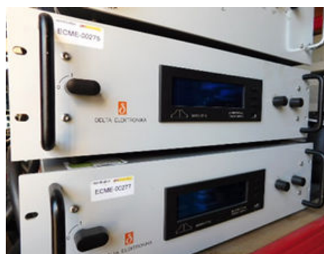
HV 2 quadrant power supply
